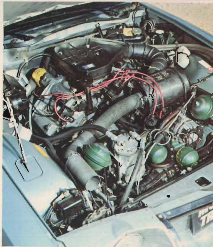
Top: French Q-ship, rocket ship, cruise ship all in one. Above: Panel member Karl Ludvigsen in SM during test trip. Right: Maserati V6 is smuggled up to firewall, preceded by 5-speed transmission, labyrinth of hydraulic equipment.
